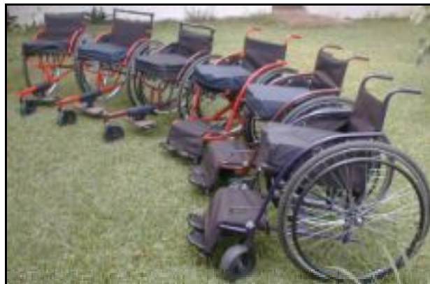
Different wheelchair designs fabricated by students
