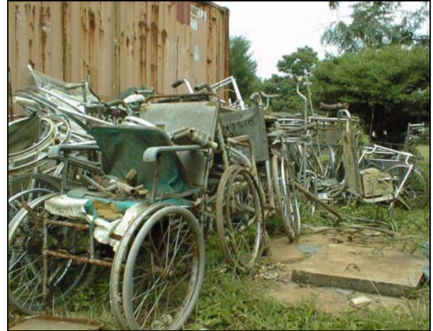
A pile of broken donated wheelchairs in Tanzania. These chairs were unable to survive the conditions in a low-income country and no spare parts were available locally.
